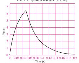
**Comments:** Note that the two parts of the response are based on two different time constants, and that the rising portion of the response changes faster (shorter time constant) than the decaying part.
