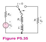
**5.36** The inductor *L* in the circuit shown in Figure P5.36 is the coil of a relay. When the current through the coil is equal to or greater than +2 mA, the relay functions. Assume steady-state conditions at t < 0. If
