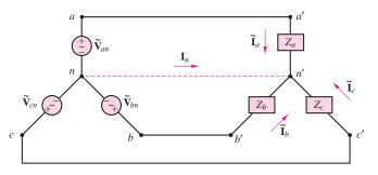
Figure 7.34 Balanced three-phase AC circuit
