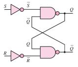
Figure 12.63 Logic gate implementation of the *RS* flip-flop
