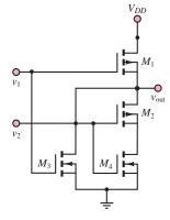
The transistors in this circuit show the substrate for each transistor connected to its respective gate. In a true CMOS IC, the substrates for the *p*-channel transistors are connected to 5 V and the substrates of the *n*-channel transistors are connected to ground.
