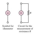
Figure 2.47 Ohmmeter and measurement of resistance
