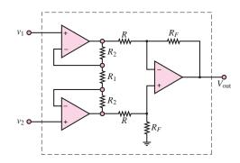
Figure 8.14 Instrumentation amplifier
