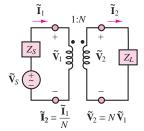
Figure 7.27 Operation of an ideal transformer
