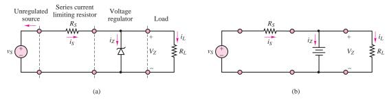
Figure 9.49 (a) A Zener diode voltage regulator; (b) simplified circuit for Zener regulator
