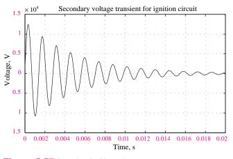
Figure 5.57 Secondary ignition voltage response
