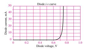
**Figure 9.8** Semiconductor diode *i*-*v* characteristic
