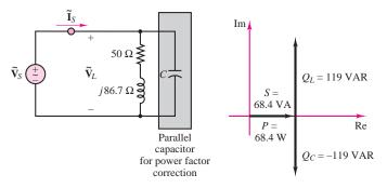
Figure 7.20 Power factor correction
