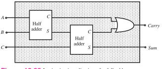
Figure 12.28 Logic circuit realization of a full adder
