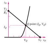
Figure 9.30 Graphical solution of equations 9.13 and 9.14
