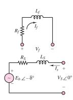
Figure 14.33 Per-phase circuit model
