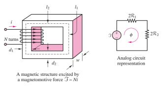
Figure 13.12 Analogy between magnetic and electric circuits
