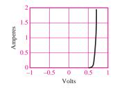
**Figure 3.72** The *i*-*v* characteristic of exponential resistor
