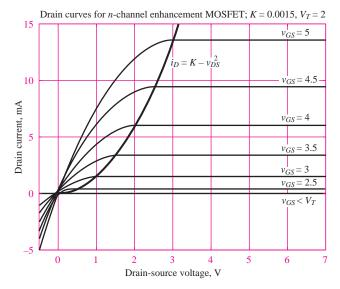
**Figure 11.5** Drain characteristic curves for a typical NMOS transistor with  $V_T = 2$  V and K = 1.5 mA/V<sup>2</sup>
