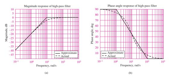
Figure 6.22 Bode plots for high-pass RC filter. (a) Magnitude response; (b) phase response
