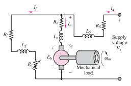
Figure 14.18 Equivalent circuit of a cumulatively compounded motor
