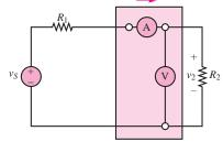
Measurement of the power dissipated in the resistor  $R_2$ :  $P_2 = v_2 i$
