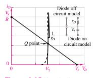
Figure 9.35 Piecewise linear diode model
