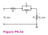
**6.33** In the filter circuit shown in Figure P6.32, derive the equation for the voltage frequency response
