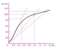
Figure 14.16 DC machine magnetization curve
