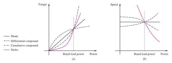
Figure 14.19 DC motor operating characteristics
