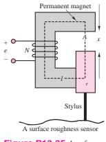
Figure P13.35 A surface roughness sensor
