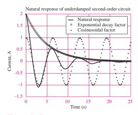
**Figure 5.45** Natural response of an underdamped second-order system for  $\alpha_1 = \alpha_2 = 1$ ;  $\zeta = 0.2$ ;  $\omega_n = 1$
