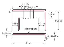
Figure 13.18 Electromagnetic structure with air gaps
