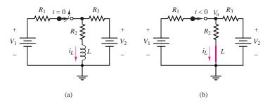
**Figure 5.10** (a) Circuit for Example 5.4; (b) same circuit a long time before the switch is opened
