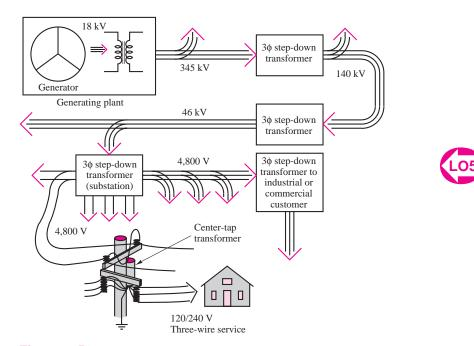
Figure 7.52 Structure of an AC power distribution network
