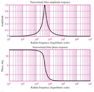
**Figure 6.20** Frequency response of narrowband bandpass filter of Example 6.7
