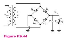
**9.45** In the full-wave power supply shown in Figure P9.44 the diodes are 1N4001
