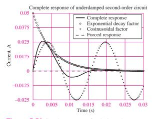
Figure 5.53 Complete response of underdamped second-order circuit
