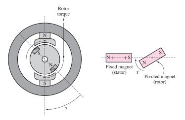
Figure 14.7 Alignment action of poles
