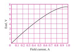
Figure 14.22 Magnetization curve for a small DC motor
