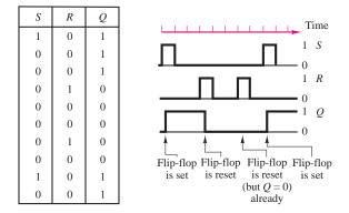
Figure 12.62 Timing diagram for the RS flip-flop
