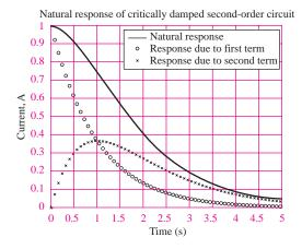
**Figure 5.44** Natural response of a critically damped second-order system for  $\alpha_1 = \alpha_2 = 1$ ;  $\zeta = 1$ ;  $\omega_n = 1$
