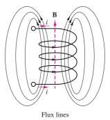
Figure 13.5 Concept of flux linkage
