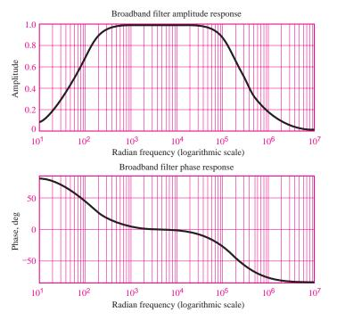
**Figure 6.19** Frequency response of broadband bandpass filter of Example 6.7
