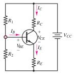
Figure 10.26 Practical BJT self-bias DC circuit the base terminal for the transistor will see the Thévenin equivalent circuit composed of the equivalent voltage source
