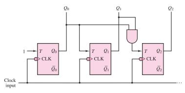
Figure 12.76 Three-bit synchronous counter
