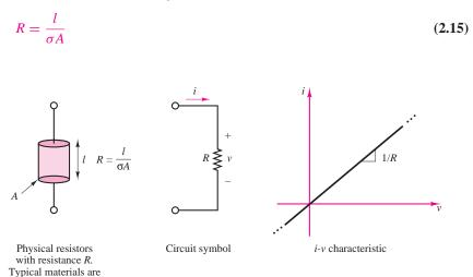
Figure 2.29 The resistance element
