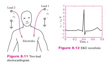
Unfortunately, the presence of electrical equipment powered by the 60-Hz, 110-V AC line current causes undesired interference at the electrode leads: the lead wires act as antennas and pick up some of the 60-Hz signal in addition to the desired EKG voltage. In effect, instead of recording the desired EKG signals  $v_1$  and  $v_2$ , the two electrodes provide the following inputs to the EKG amplifier, shown in Figure 8.13:
