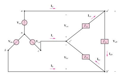
Figure 7.40 Balanced wye generators with balanced delta load
