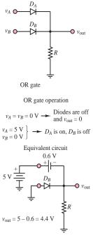
Figure 10.29 Diode OR gate
