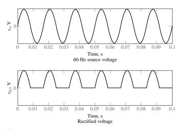
Figure 9.21 Ideal diode rectifier input and output voltages
