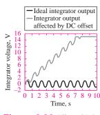
Figure 8.36 Effect of DC offset on integrator
