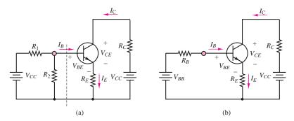
Figure 10.27 DC self-bias circuit represented in equivalent-circuit form
