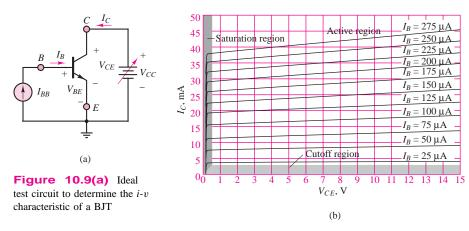
Figure 10.9(b) The collector-emitter output characteristics of a BJT
