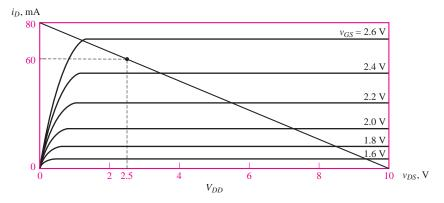
Figure 11.19 Drain curves for MOSFET of Figure 11.18
