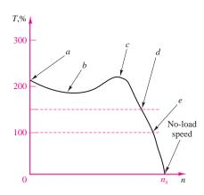
Figure 14.42 Performance curve for induction motor
