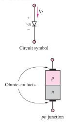
Figure 9.9 Semiconductor diode circuit symbol
