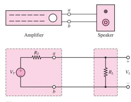
Figure 3.71 A simplified model of an audio system
