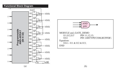
**Figure 12.59** (a) The ispGAL16V8 connection diagram; (b) sample code for AND function (for ispGAL16V8).
