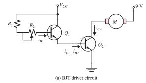
Figure 10.17 Motor drive circuit
