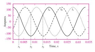
Figure 14.26 Three-phase stator winding currents
