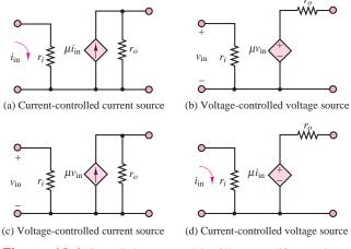
Figure 10.1 Controlled source models of linear amplifier transistor operation
