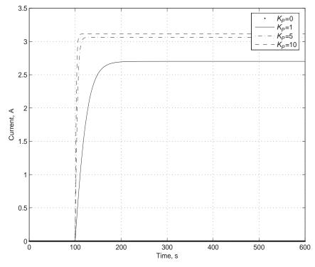
Figure 8.18 (e) Power amplifier output current for various proportional gain,  $K_p$
