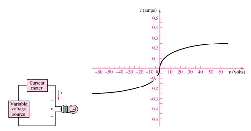
Figure 2.27 Volt-ampere characteristic of a tungsten lightbulb
