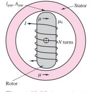
Figure 13.22 Cross-sectional view of synchronous motor
