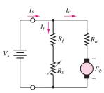
Figure 14.21 Shunt motor
