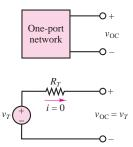
Figure 3.43 Equivalence of open-circuit and Thévenin voltage
