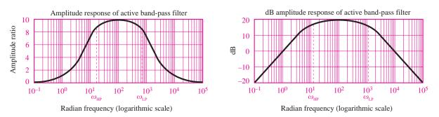
Figure 8.26 Normalized amplitude response of active bandpass filter
