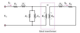
Figure 14.38 Circuit model for induction machine
