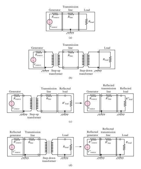
**Figure 7.31** Electric power transmission: (a) direct power transmission; (b) power transmission with transformers; (c) equivalent circuit seen by generator; (d) equivalent circuit seen by load
