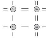
Figure 9.1 Lattice structure of silicon, with four valence electrons
