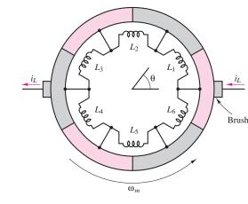
Figure 14.13 Rotor winding and commutator
