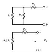
Figure 3.37 Equivalent resistance seen by the load
