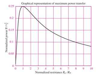
Figure 3.69 Graphical representation of maximum power transfer
