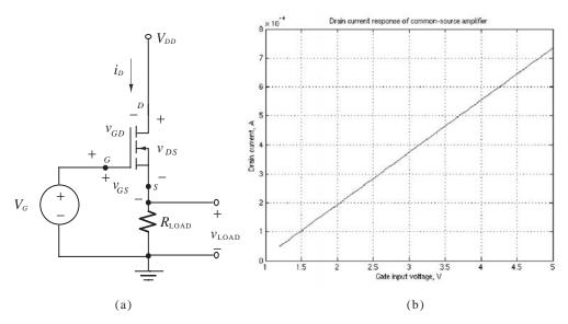
**Figure 11.13** (a) Source-follower MOSFET amplifier. (b) Drain current response for a 100- $\Omega$  load when K = 0.018 and  $V_T = 1.2$  V
