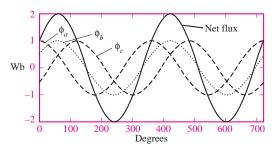
Figure 14.27 Flux distribution in a three-phase stator winding as a function of angle of rotation
