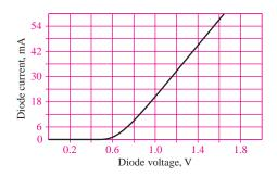
Figure 9.32 The 1N914 diode *i*-v curve
