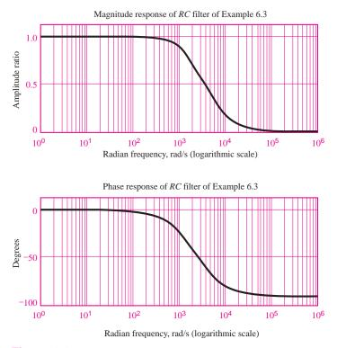
Figure 6.9 Response of *RC* filter of Example 6.3
