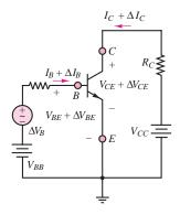
**Figure 10.21** Circuit illustrating the amplification effect in a BJT
