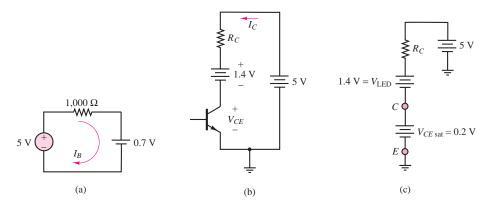
**Figure 10.15** (a) *BE* circuit for LED driver; (b) equivalent collector circuit of LED driver, assuming that the BJT is in the linear active region; (c) LED driver equivalent collector circuit, assuming that the BJT is in the saturation region
