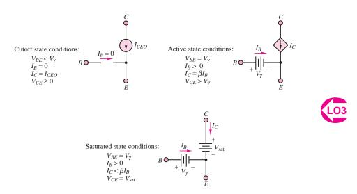
Figure 10.12 An npn BJT large-signal model
