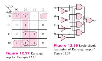
The implementation of the above function with logic gates is shown in Figure 12.38.
