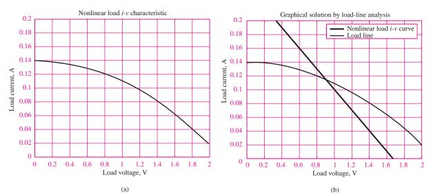
The solution for  $v_x$  and  $i_x$  occurs at the intersection of the device and load-line characteristics:  $i_x \approx 0.12 \text{ A}, v_x \approx 0.9 \text{ V}.$
