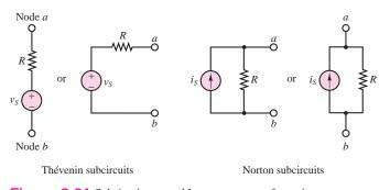
Figure 3.61 Subcircuits amenable to source transformation
