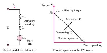
Figure 14.20 Circuit model and torque-speed curve of PM motor
