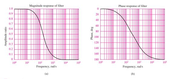
Figure 6.12 Frequency response of filter of Example 6.5. (a) Magnitude response; (b) phase response
