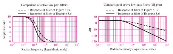
Figure 8.28 Comparison of first- and second-order active filters
