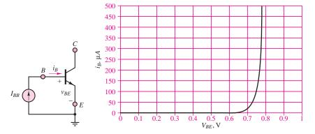
Figure 10.8 The BE junction open-collector curve
