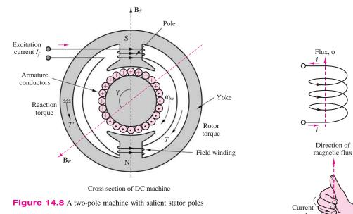
To understand magnetic polarity, we need to consider the direction of the magnetic field in a coil carrying current. Figure 14.9 shows how the *right-hand rule* can be employed to determine the direction of the magnetic flux. If one were to grasp the rule
