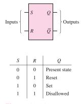
**Figure 12.61** *RS* flip-flop symbol and truth table
