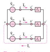
Figure 7.36 Balanced three-phase AC circuit (redrawn)
