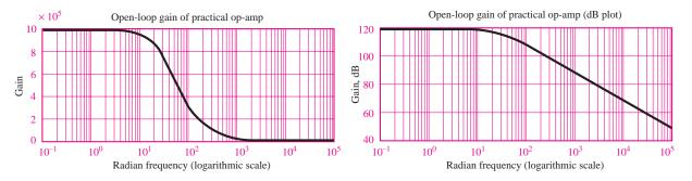
Figure 8.37 Open-loop gain of practical op-amp
