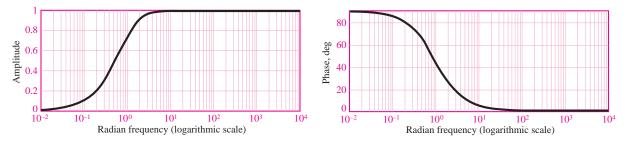
Figure 6.14 Frequency response of a high-pass filter
