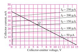
**Figure 10.19** Load-line analysis of a simplified BJT amplifier
