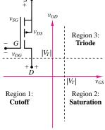
Figure 11.11 Regions of operation of PMOS transistor
