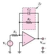
Figure 8.20 Active low-pass filter
