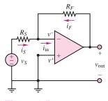
Figure 8.5 Inverting amplifier
