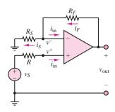
Figure 8.8 Noninverting amplifier
