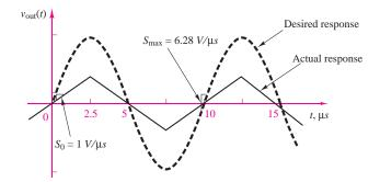
Figure 8.46 Distortion introduced by slew rate limit
