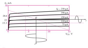
Figure 10.22 Amplification of sinusoidal oscillations in a BJT
