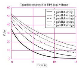
Figure 5.35 Transient response of supercapacitor circuit
