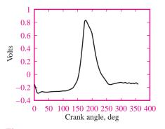
Figure 12.1 Voltage analog of internal combustion engine in-cylinder pressure
