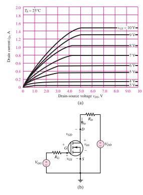
if  $V_{GG} = 7$  V;  $V_{DD} = 10$  V; and  $R_D = 5 \Omega$ . In what region is the transistor operating?
