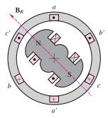
Figure 14.10 Magnetic field in a salient rotor winding
