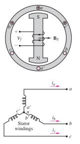
Figure 14.25 Two-pole three-phase stator
