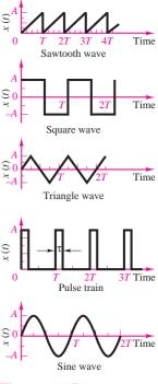
Figure 4.15 Periodic signal waveforms
