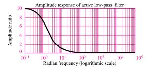
Figure 8.22 Normalized response of active low-pass filter
