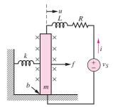
**Figure 13.46** A more realistic representation of the transducer of Figure 13.45
