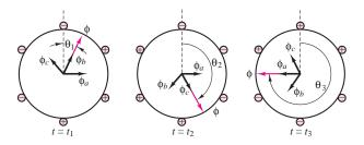
Figure 14.28 Rotating flux in a three-phase machine
