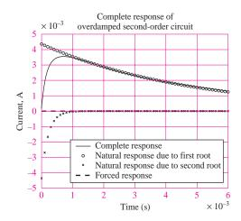
Figure 5.49 Complete response of overdamped second-order circuit
