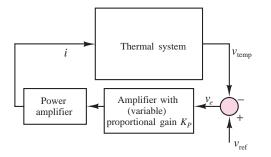
Figure 8.18 (b) Block diagram of control system
