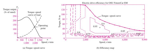
Figure 14.4 Torque–speed and efficiency curves for an electric motor
