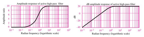
Figure 8.24 Normalized response of active high-pass filter
