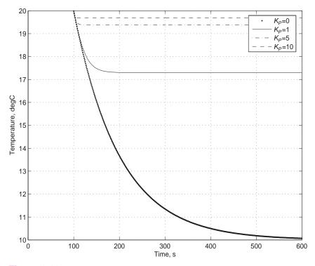
Figure 8.18 (d) Response of thermal system for various values of proportional gain,  $K_p$
