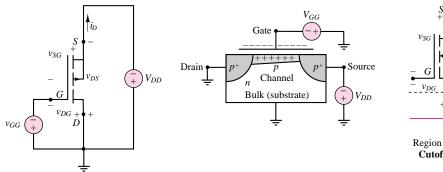
**Figure 11.10** The *p*-channel enhancement-mode field-effect transistor (PMOS)
