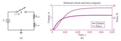
Figure 13.37 Solenoid equivalent electric circuit and step response
