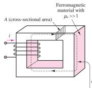
Mean path of magnetic flux lines (note how the path of the flux is enclosed within the magnetic structure)
