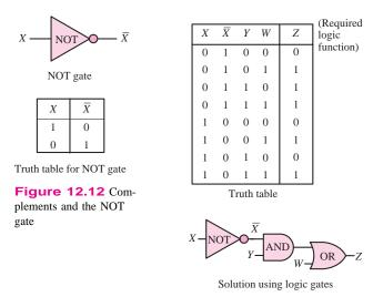
Figure 12.13 Solution of a logic problem using logic gates
