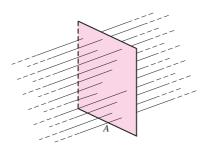
Figure 13.3 Magnetic flux lines crossing a surface
