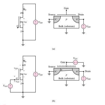
**Figure 11.3** Channel formation in NMOS transistor: (a) With no external gate voltage, the source-substrate and substrate-drain junctions are both reverse-biased, and no conduction occurs; (b) when a gate voltage is applied, charge-carrying electrons are drawn between the source and drain regions to form a conducting channel.
