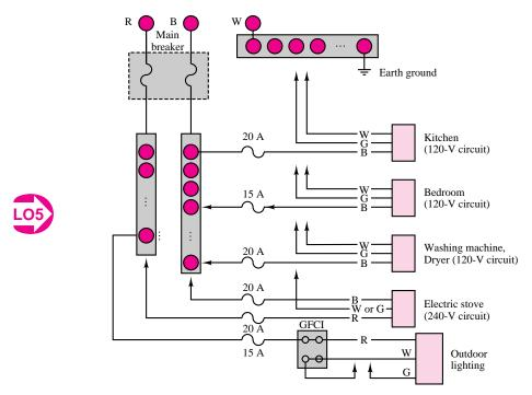
Figure 7.46 A typical residential wiring arrangement
