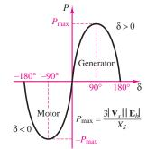
Figure 14.35 Power versus power angle for a synchronous machine
