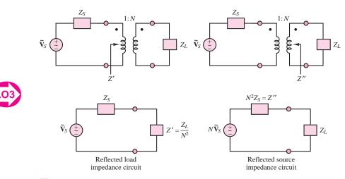
Figure 7.28 Impedance reflection across a transformer
