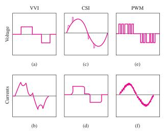
Figure 14.46 Typical adjustable-frequency controller voltage and current waveforms (*Courtesy: Rockwell Automation, Reliance Electric.*)
