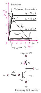
Figure 10.30 BJT switching characteristic
