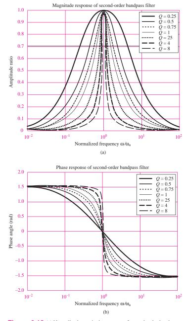
**Figure 6.18** (a) Normalized magnitude response of second-order bandpass filter; (b) normalized phase response of second-order bandpass filter
