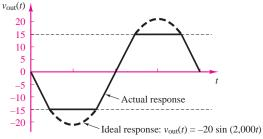
have you ever wondered why rock guitar has a characteristic sound that is very different from the sound of classical or jazz guitar? The reason is that the "rock sound" is obtained by overamplifying the signal, attempting to exceed the voltage supply limits, and causing clipping similar in quality to the distortion introduced by voltage supply limits in an op-amp. This clipping broadens the spectral content of each tone and causes the sound to be distorted.
