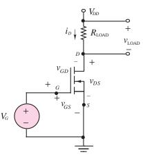
Figure 11.12 Common-source MOSFET amplifier
