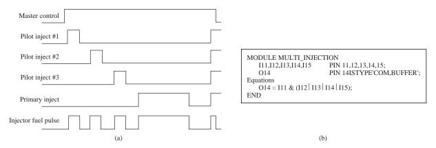
Figure 12.60 (a) Injector timing sequence; (b) sample code for multiple-injection sequence
