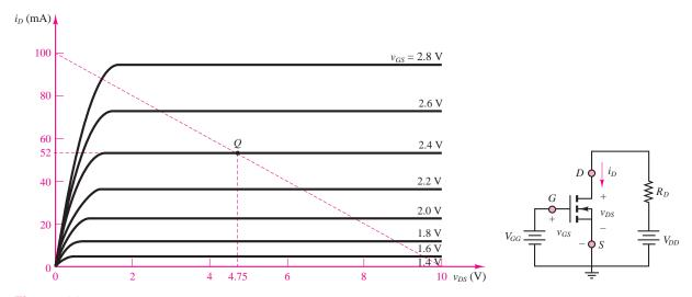
Figure 11.7 The *n*-channel enhancement MOSFET circuit and drain characteristic for Example 11.2
