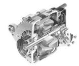
Figure 14.32 Automotive alternator (*Courtesy: Delphi Automotive Systems.*)
