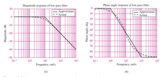
**Figure 6.21** Bode plots for low-pass *RC* filter; the frequency variable is normalized to  $\omega/\omega_0$ . (a) Magnitude response; (b) phase response
