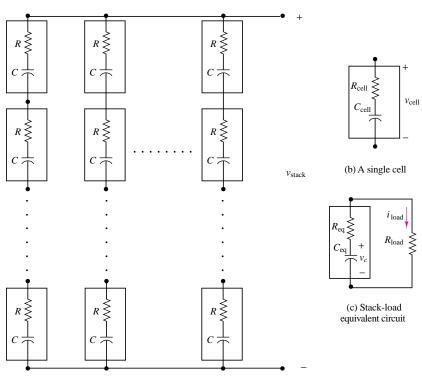
(a) An ultracapacitor stack
