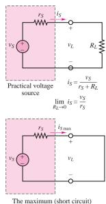
The maximum (short circuit) current which can be supplied by a practical voltage source is
