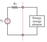
Figure 5.24 Equivalentcircuit representation of first-order circuits
