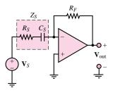
Figure 8.23 Active high-pass filter
