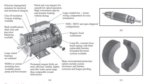
**Figure 14.12** (a) DC machine; (b) rotor; (c) permanent-magnet stator (*Photos* © 2005, *Rockwell Automation. All rights reserved. Used with permission.*)
