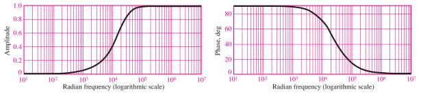
Figure 6.15 Response of high-pass filter of Example 6.6
