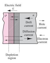
**Figure 9.6** Drift and diffusion currents in a *pn* junction
