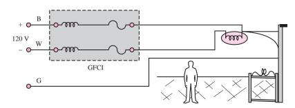
Figure 7.51 Use of a GFCI in a potentially hazardous setting
