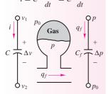
Figure 4.1 Analogy between electrical and fluid capacitance
