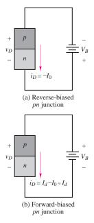
Figure 9.7 Forwardand reverse-biased *pn* junctions
