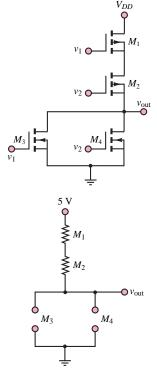
With both  $v_1$  and  $v_2$  at 0 V,  $M_3$  and  $M_4$  will be turned off (in cutoff), since  $v_{GS}$  is less than  $V_T(0 \vee < 1.7 \vee)$ . Both  $M_1$  and  $M_2$  will be turned on, since the gate-to-source voltages will be greater than  $V_T$ .
