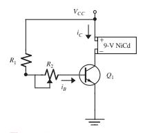
Figure 10.16 Simple battery charging circuit
