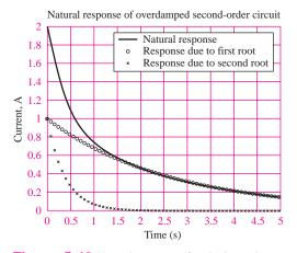
**Figure 5.43** Natural response of underdamped second-order system for  $\alpha_1 = \alpha_2 = 1$ ;  $\zeta = 1.5$ ;  $\omega_n = 1$
