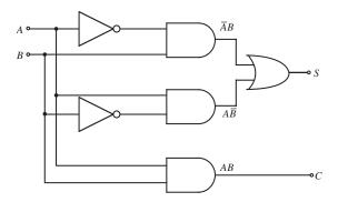
Figure 12.27 Logic circuit realization of a half adder
