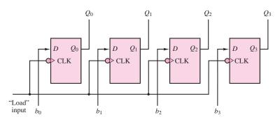
Figure 12.78 A 4-bit parallel register
