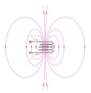
Figure 13.9 Magnetic flux lines in the vicinity of a current-carrying coil
