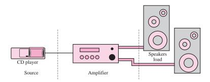
Figure 8.1 Amplifier in audio system
