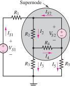
Figure 2.14 Application of KCL with a supernode
