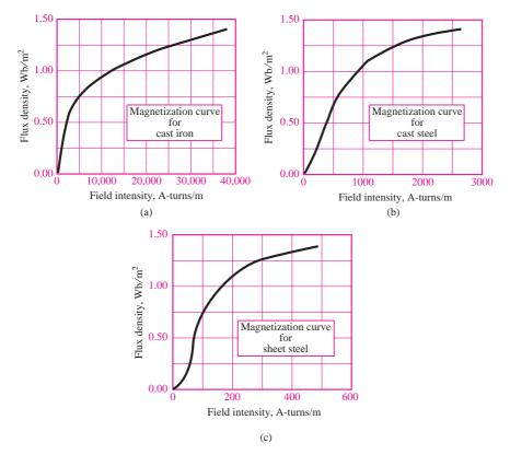
**Figure 13.28** (a) Magnetization curve for cast iron; (b) magnetization curve for cast steel; (c) magnetization curve for sheet steel
