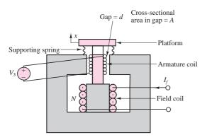
Figure P13.49 Electrodynamic shaker
