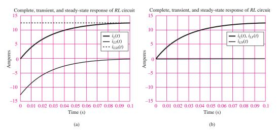
Figure 5.23 Transient response of electric motor: (a) steady-state and transient responses; (b) natural and forced responses
