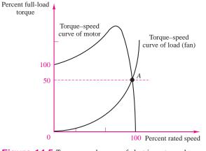
Figure 14.5 Torque–speed curves of electric motor and load
