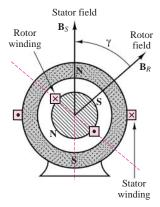
Figure 14.1 A rotating electric machine
