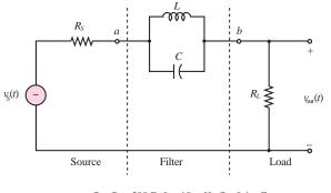
$R_{\rm S} = R_{\rm L} = 500 \,\Omega; L = 10 \, mH; \, C = 0.1 \, \mu F$
