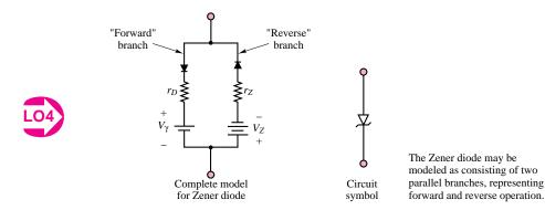
Figure 9.48 Complete model for Zener diode
