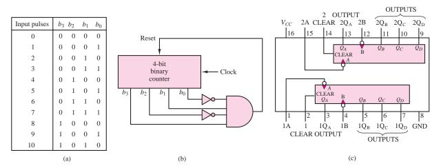
Figure 12.71 Decade counter: (a) counting sequence; (b) functional diagram; and (c) IC schematic
