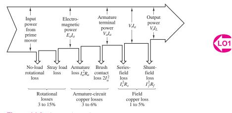
Figure 14.3a Generator losses, direct current
