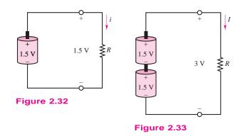
**Analysis:** We first need to obtain an expression for resistor power dissipation as a function of its resistance. We know that P = VI and that V = IR. Thus, the power dissipated by any resistor is
