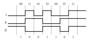
**Comments:** How would the timing diagram change if the initial state of the flip-flop were  $Q_0 = 1$ ?
