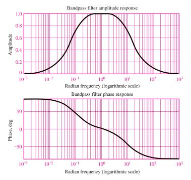
Figure 6.17 Frequency responses of RLC bandpass filter
