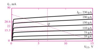
Figure 10.25 Operating point on the characteristic curve
