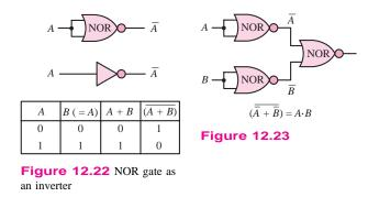
**Comments:** NOR gates naturally implement functions that contain complemented sums. Gates that employ negative logic are a natural consequence of the inverting characteristics of transistor switches (refer to Section 10.5). Thus, one should expect that NOR (and NAND) gates are very commonly employed in practice.
