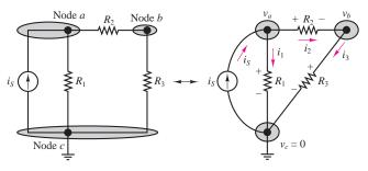
Figure 3.4 Illustration of node analysis
