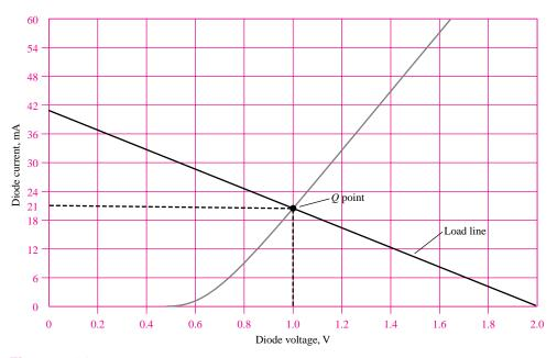
Figure 9.34 Superposition of load line and diode *i*-v curve
