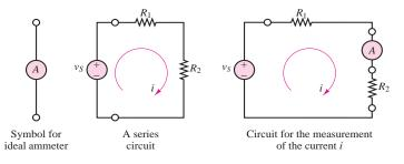
Figure 2.48 Measurement of current
