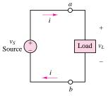
Figure 2.17 Sources and loads in an electric circuit
