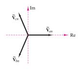
**Figure 7.35** Positive, or *abc*, sequence for balanced three-phase voltages
