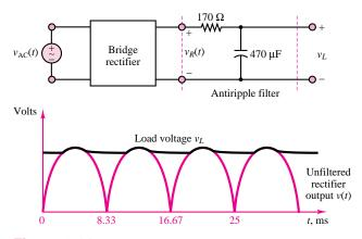
Figure 9.44 Bridge rectifier with filter circuit
