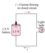
Figure 2.10 A simple electric circuit
