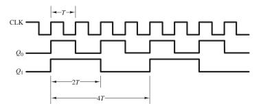
Figure 12.75 Divider circuit timing diagram
