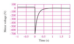
Figure 5.33 Motor voltage transient response
