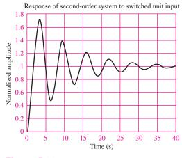
**Figure 5.39** Response of switched second-order system with  $K_S = 1$ ,  $\omega_n = 1$ , and  $\zeta = 0.1$
