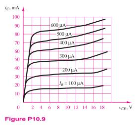
*Hint:* A reasonable approximation for the power dissipated at the collector is the product of the collector voltage and current  $P = I_C V_{CE}$ , where P is the permissible power dissipation,  $I_C$  is the quiescent collector current, and  $V_{CE}$  is the operating point collector-emitter voltage.
