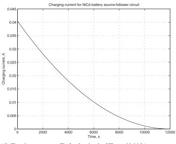
(d) Charging current profile for the circuit of Figure 11.14(b)
