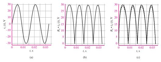
**Figure 9.43** (a) Unrectified source voltage; (b) rectified load voltage (ideal diodes); (c) rectified load voltage (ideal and offset diodes)
