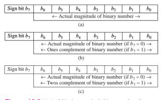
**Figure 12.8** (a) An 8-bit sign-magnitude binary number; (b) an 8-bit ones complement binary number; (c) an 8-bit twos complement binary number
