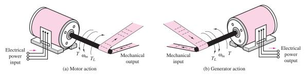
Figure 14.6 Generator and motor action in an electric machine
