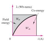
**Figure 13.7** Relationship between flux linkage, current, energy, and co-energy
