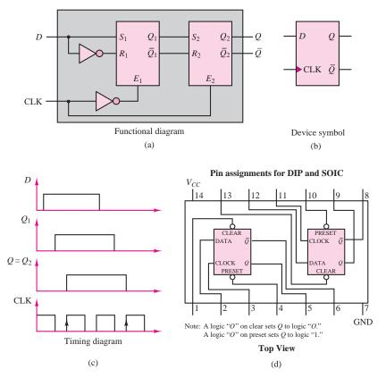
**Figure 12.66** The *D* flip-flop: (a) functional diagram; (b) symbol; (c) timing waveforms; and (d) IC schematic
