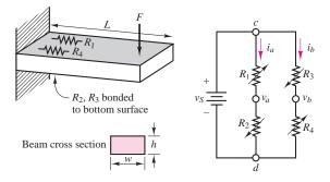
Figure 2.44 A force-measuring instrument.
