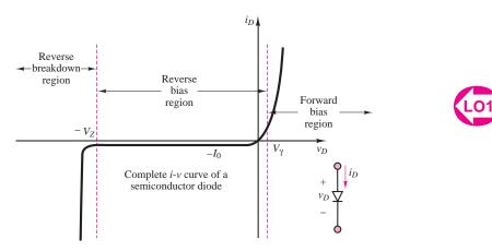
Figure 9.10 The *i*-v characteristic of the semiconductor diode
