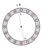
Figure 14.11 Magnetic field of stator
