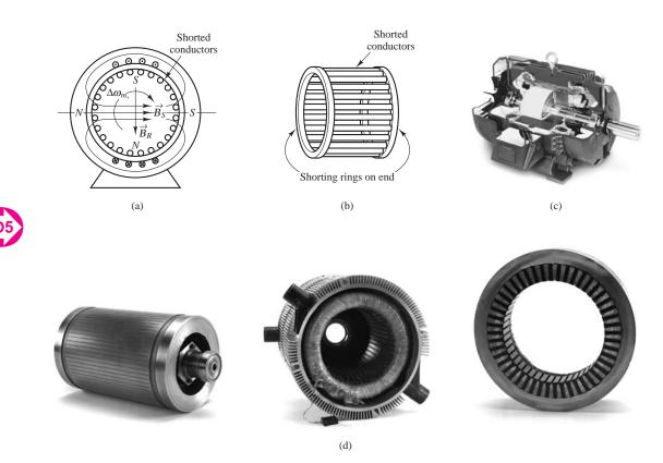
Figure 14.37 (a) Squirrel cage induction motor; (b) conductors in rotor; (c) photograph of squirrel cage induction motor; (d) views of Smokin' Buckeye motor: rotor, stator, and cross section of stator (*Photos Courtesy: David H. Koether Photography.*)
