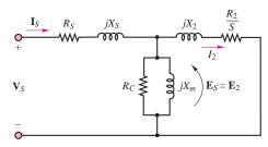
Figure 14.40 Equivalent circuit of an induction machine
