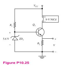
**10.26** The circuit of Figure P10.26 is a variation of the battery charging circuit of Problem 10.25. Analyze the operation of the circuit and explain how this circuit will provide a decreasing charging current (taper current cycle) until the NiCd battery is fully charged (10.4 V—see note in Example 10.5). Choose appropriate values of  $V_{CC}$  and  $R_1$  that would result in a practical design. Use standard resistor values.
