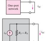
Figure 3.53 Illustration of Norton equivalent circuit
