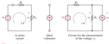
Figure 2.49 Measurement of voltage
