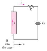
Figure 13.45 Motor and generator action in an ideal transducer
