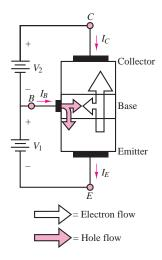
When the *BC* junction is reversebiased, the electrons from the emitter region are swept across the base into the collector.
