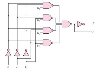
Figure 12.53 Internal structure of the 4-to-1 MUX
