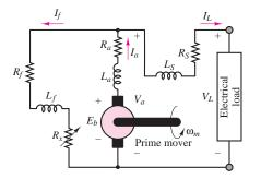
Figure 14.17 Compound generator circuit model
