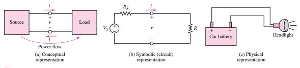
Figure 2.2 Various representations of an electrical system
