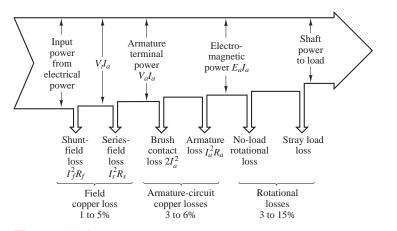
Figure 14.3b Motor losses, direct current
