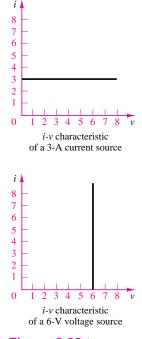
Figure 2.28 *i*-v characteristics of ideal sources
