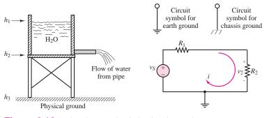
Figure 2.18 Analogy between electrical and earth ground
