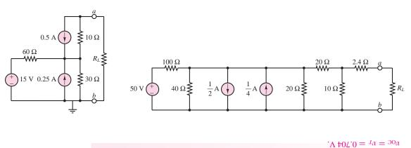
Find the Thévenin equivalent circuit for the circuit in the figure on the right.
