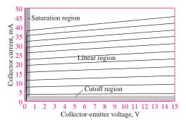
Figure 10.13 BJT collector characteristic
