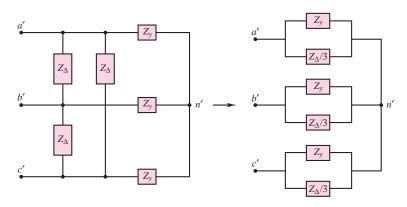
Figure 7.42 Conversion of delta load to equivalent wye load
