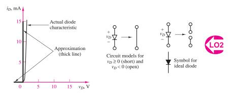
Figure 9.11 Large-signal on/off diode model
