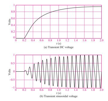
Figure 5.1 Examples of transient response
