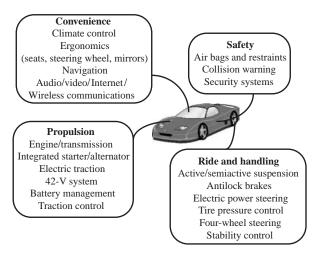
Figure 1.2 Electrical engineering systems in the automobile
