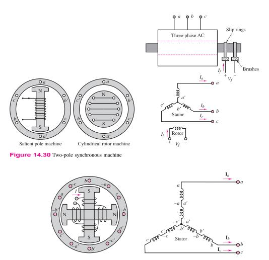
Figure 14.31 Four-pole three-phase alternator
