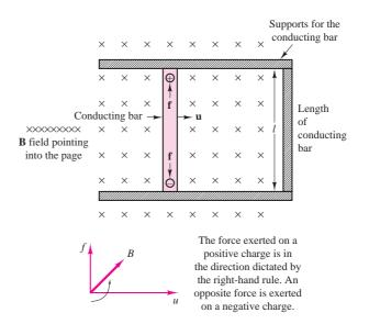
Figure 13.42 A simple electromechanical motion transducer
