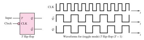
Figure 12.69 The T flip-flop symbol and timing waveforms
