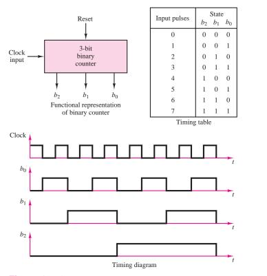
Figure 12.70 Binary up counter functional representation, state table, and timing waveforms
