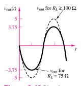
Figure 8.48 Distortion introduced by short-circuit current limit
