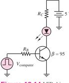
Figure 10.14 LED driver circuit
