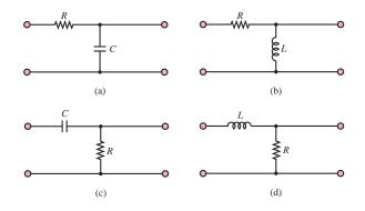
Show that it is possible to obtain a high-pass filter response simply by substituting an inductor for the capacitor in the circuit of Figure 6.7. Derive the frequency response for the circuit.
