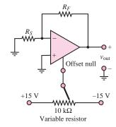
Figure 8.43 Output offset voltage adjustment
