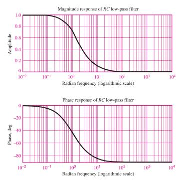
Figure 6.8 Magnitude and phase response plots for RC filter
