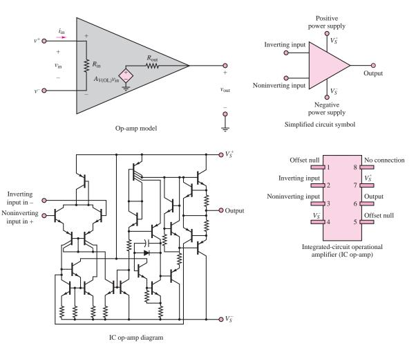
Figure 8.4 Operational amplifier model symbols, and circuit diagram
