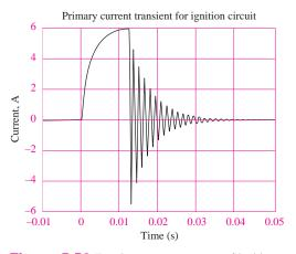
Figure 5.56 Transient current response of ignition current
