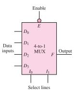
Figure 12.54 Functional diagram of four-input MUX
