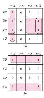
Figure 12.33 Four- and eight-cell subcubes for an arbitrary logic function
