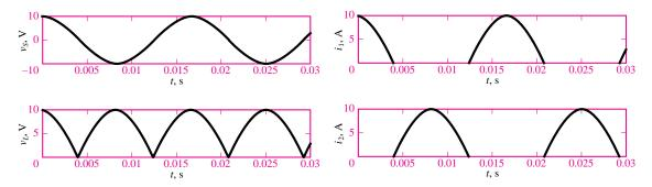
**Figure 9.40** Full-wave rectifier current and voltage waveforms ( $R_L = 1 \Omega$ )
