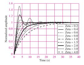
**Figure 5.40** Response of switched second-order system with  $K_S = 1$ ,  $\omega_n = 1$ , and  $\zeta$  ranging from 0.2 to 4
