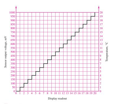
Figure 12.2 Digital representation of an analog signal
