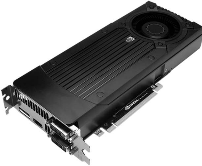
Figure 5.1 A typical NVIDIA GPU card. For example, NVIDIA Tesla C1060 – number of streaming multiprocessors (SMs): 30; number of cores (or streaming processors, SPs) per SM: 8; total number of cores: 30 \times 8 = 240 ; clock rate: 1.3 GHz; global memory: 4 GB; shared memory per SM: 16 KB.
